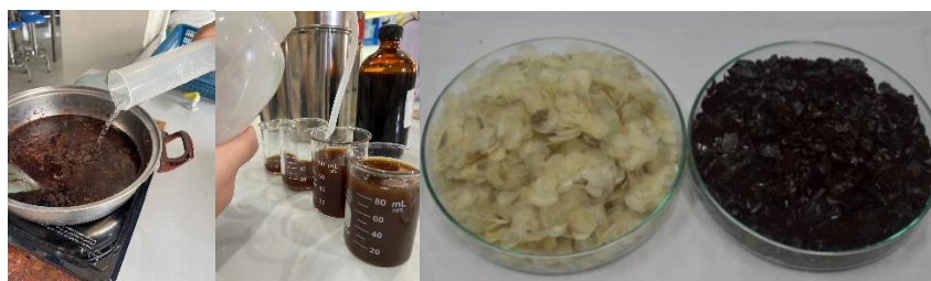
Figure 2. biochar adsorbent (0.1 g) was introduced into 50 mL of ethanolic extract prepared across a range of initial concentrations. The mixture was agitated for 24 hours using a stir plate at room temperature (25°C) to ensure complete equilibration between the liquid and solid phases.
