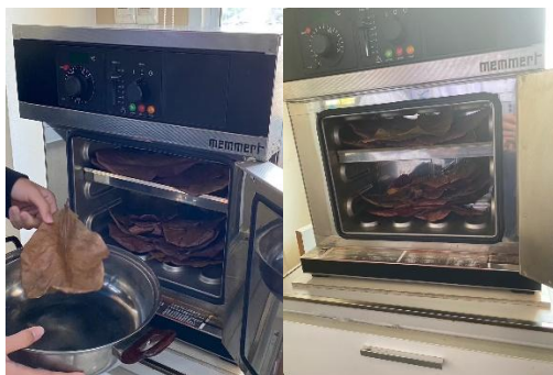
Figure 1. Dried T. catappa leaves were washed, oven-dried, and ground into a powder. This powder was then mixed with a 70% ethanol solution and extracted at 60°C for 2 hours.
