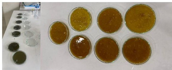
Figure 3. The biochar-adsorbed extract was introduced into phosphate-buffered saline (PBS) within a sterile Petri dish. The system was incubated at 37°C to simulate the physiological environment of a wound.
