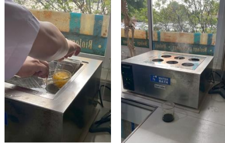
Picture 2 shows boiling fibroin in a calcium solution. Chloric ( \text{CaCl}_2 ) with 70% ethanol
