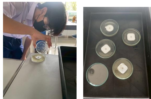
Picture 24 Display: Place the pad electrode into the gel While still liquid.
