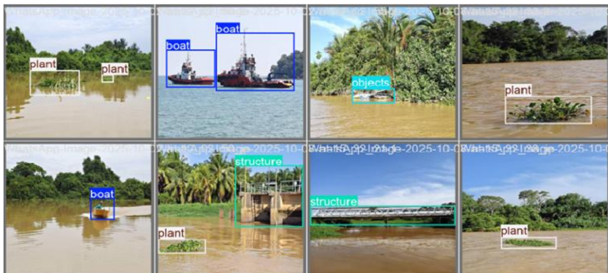
Figure 2. Example of annotated dataset with four maritime obstacle classes
