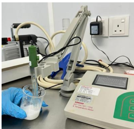
Figure 5: The pH meter for pH measurements of the sunscreen formulation
