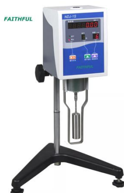
Figure 4: Rotational viscometer for viscosity measurement of the sunscreen formulations
